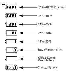
Figure 2-9 Battery Charge Status
